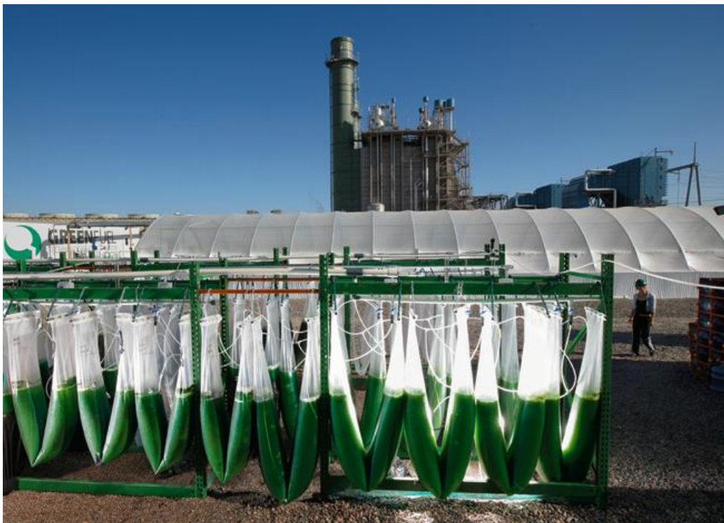
High hopes hang on bags of algae outside the Redhawk power plant near Phoenix. Researchers say the fast-growing green scum, fed by power plant exhaust, could soak up carbon dioxide while cranking out 5,000 gallons of biodiesel an acre each year—at least in theory.
